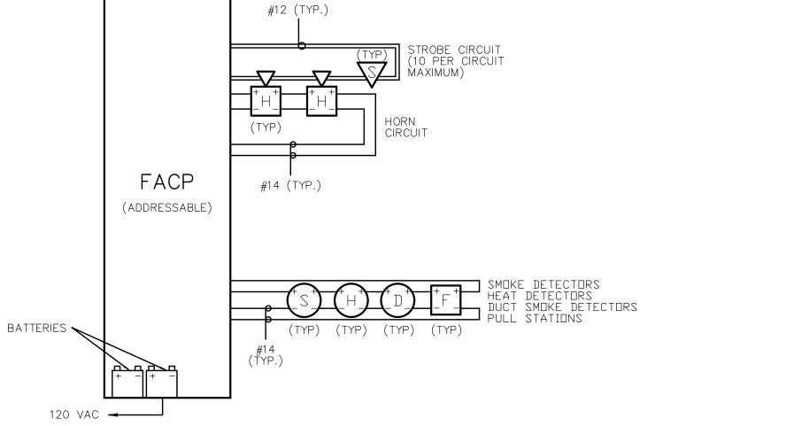
THE INTENT OF THIS RISER IS GENERAL WIRING FOR DESIGN UNLY. VERIFY EXACT REQUIREMENTS AND COMPLY WITH MANUFACTURERS RECOMMENDATIONS FOR ACTUAL EQUIPMENT FURNISHED.
